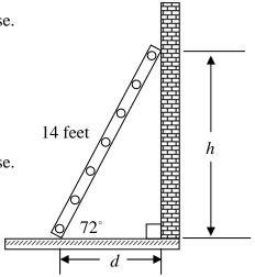
(b) Determine the height, *h*, the ladder reaches up the side of the house. Round to the nearest foot. 4. A 625 foot long wire is attached to the top of a tower. If the wire makes an angle of 65° with the ground, how tall is the tower? Round your answer to the *nearest tenth* of a foot.
